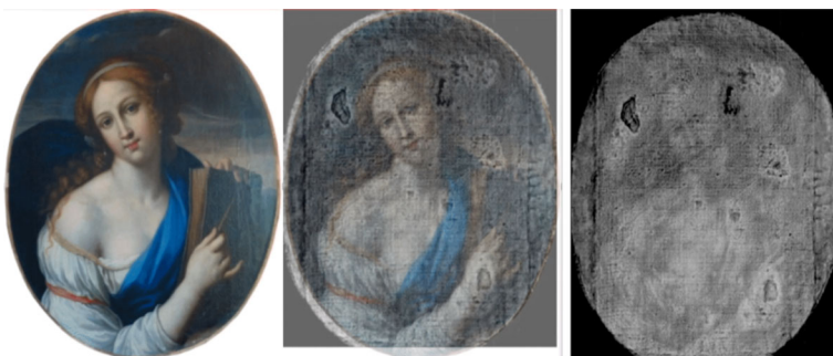
Fig. 3 On the left : photography of the painting with white light. We can observe at the right of the painting some cracks. On the right : 300-GHz reflection image of the painting. Center : image fusion between visible and millimeter wave. We note the excellent correlation between both and the precise localization of the different defects
