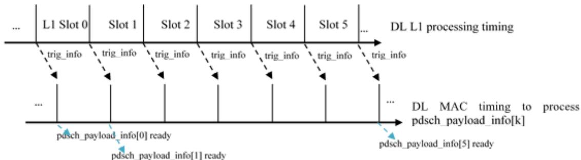
**Figure 6-75 L1/L2 Interface DL Data Processing Procedure**
