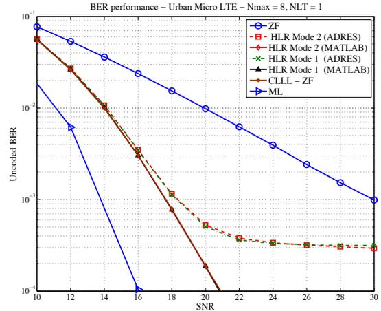
Figure 3: Unencoded BER of a 4x4 16-QAM MIMO system, Urban micro LTE channel at Speed = 3 km/h LR algorithms with ZF
