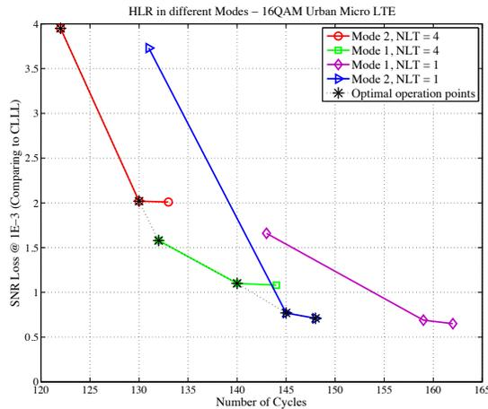
Figure 4: 4x4 16-QAM MIMO system, Performance - Cycles Tradeoff curves
