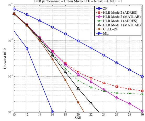
Figure 2: Unencoded BER of a 4x4 16-QAM MIMO system, Urban micro LTE channel at Speed = 3 km/h LR algorithms with ZF
