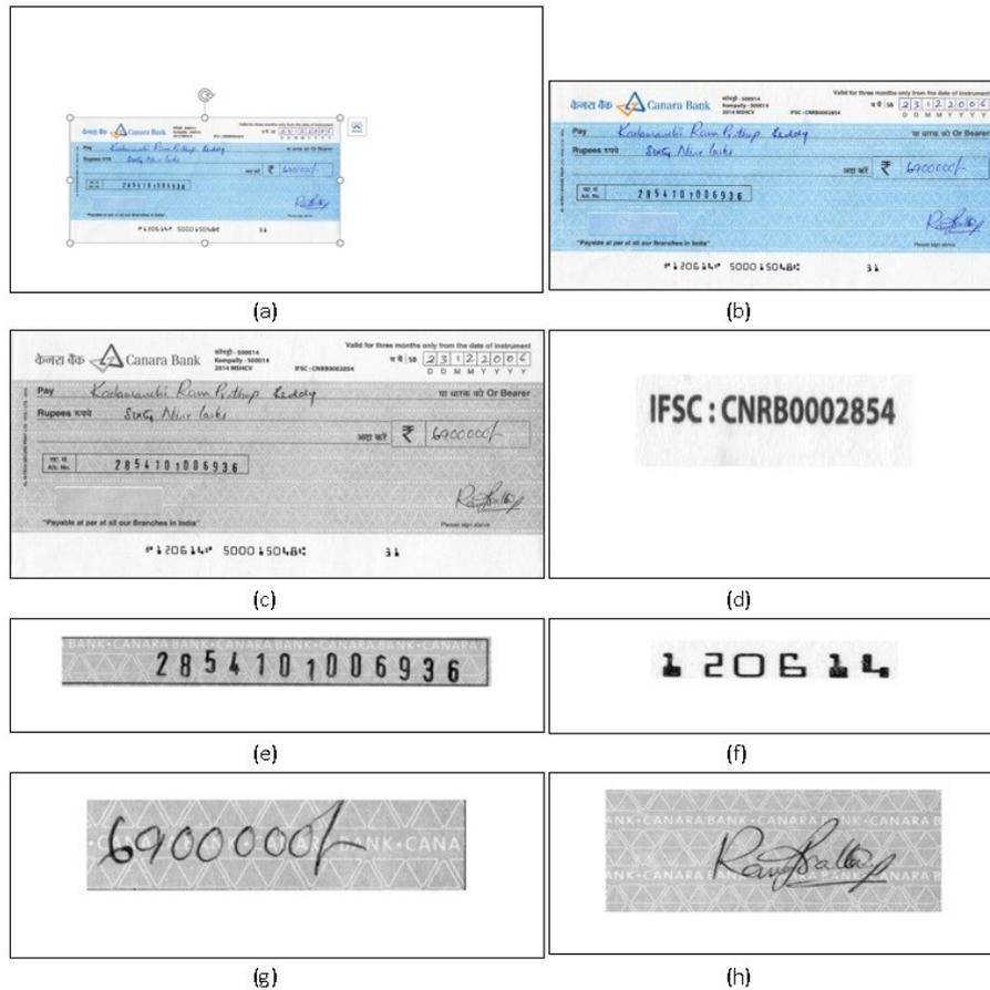
**Fig. 14** Segmentation of a bank cheque image: (a) Original scanned cheque, (b) cropped cheque leaflet, (c) gray-scale cheque image, (d) IFS code, (e) account number, (f) cheque number, (g) courtesy amount, and (h) signature.
