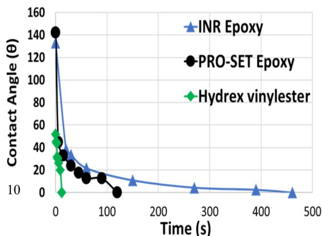
Fig. 4. Effect of Resin on the Contact Angle Change over Time for the three resin systems investigated: INR Epoxy, PRO-SET Epoxy and Hydrex Vinylester.
