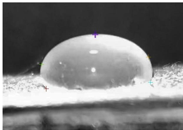
**Fig. 1.** Sample image of a resin drop on silk preform used to measure silk/resin contact angle via *ImageJ* software.
