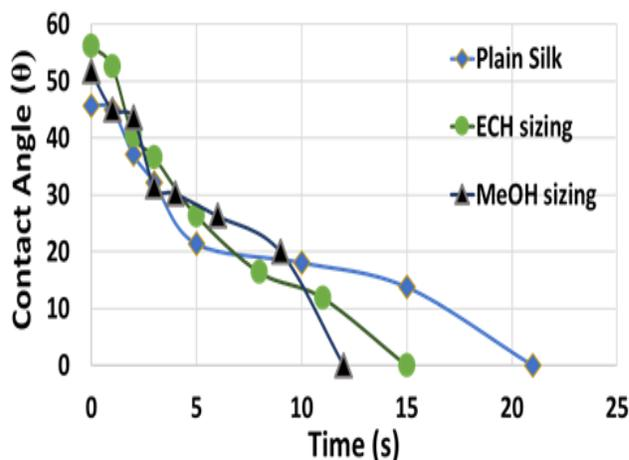
Fig. 3. Effect of Silk Treatment on the Contact Angle Change over Time for Hydrex Vinylester resin.
