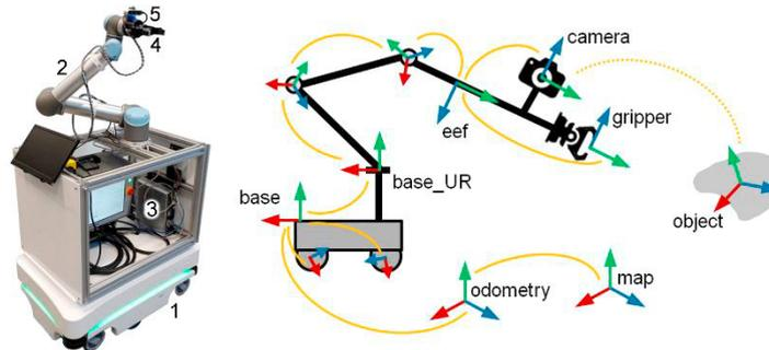
Fig. 4. Use case example: adaptive mobile manipulator including frames and kinematic structure.
