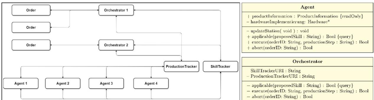
Fig. 1. Communication architecture of the UAS TW Digital Factory.
