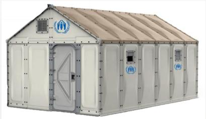
**Refuge Housing Unit**: 3 years durability; steel frame, polyolefin foam panels, UV stabilized polymer plastic (doors and windows), woven high-density polyethylene fibers (floor)
