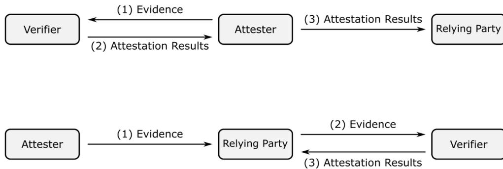
**Figure 13, the passport (top) and background-check communication model (bottom).**
