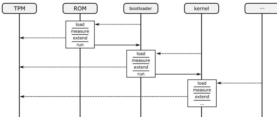
Figure 7, example of a TPM measured boot.
