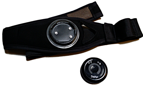
Figure 2. The Zephyr BioHarness sensor with its belt
