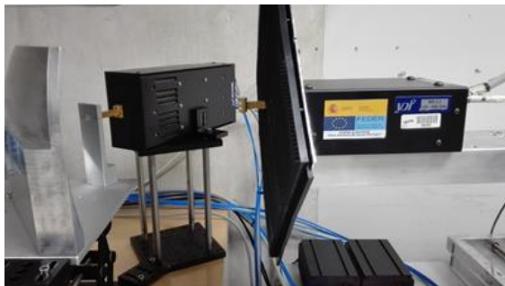
Planar near field measurement system with 330 GHz to 500 GHz frequency head extenders.
