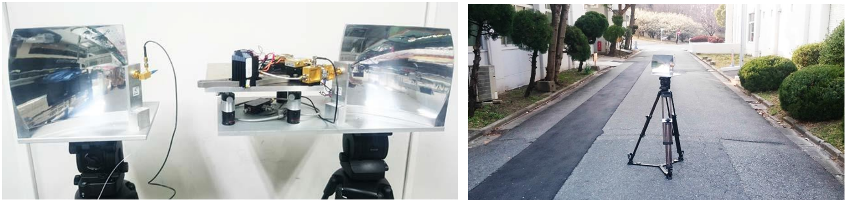
Photograph of the transmitter and receiver, which are supported by tripods.
