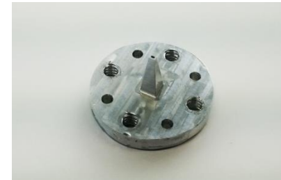
10 mm length Near field probe.
