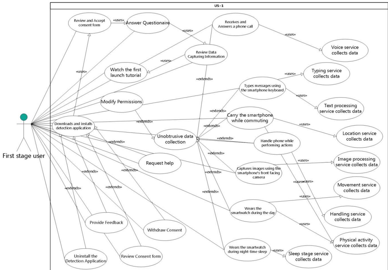
Fig. 3. The use cases and the actors in US-1 as a UML use case diagram.
