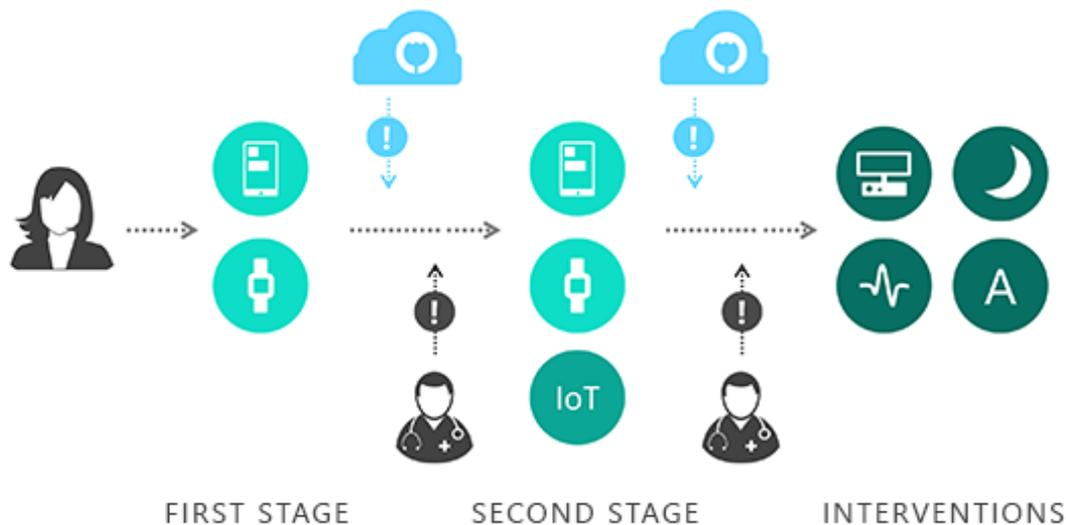
Fig. 2. The i-PROGNOSIS system concept includes two stages for PD detection based on smartphone, smartwatch and internet-of-things (IoT) user interaction and the interventions stage (serious games, nocturnal and assistive interventions, as well as monitoring). Besides, the i-PROGNOSIS automated indication of a user's behavioural change related to PD, the role of the physician is crucial regarding the validation of the indication and the transition from one stage to the next one.
