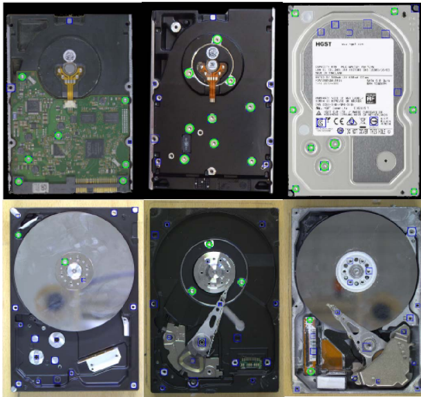
Fig. 7. Sample outputs of the pipeline. Blue rectangles show the candidates generated by Hough Transform and the green circles refer to the true positives predicted by the integrated model. Our scheme is robust to different backgrounds and to different illumination. In all of the images above, the screws were detected correctly.
