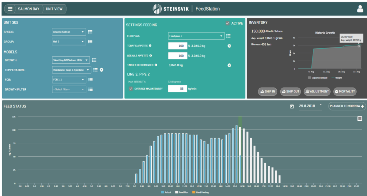
Figure 4: Control screen for the Steinsvik automation program for aquaculture farms.
