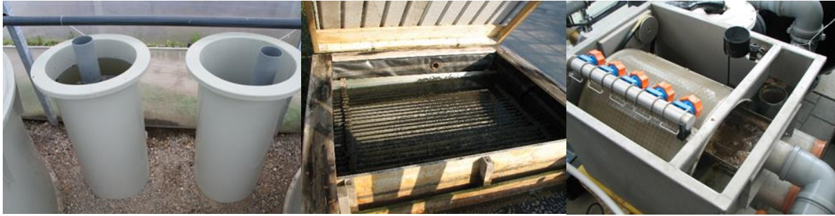
Figure 11. Different solids removal devices: (left) sludge trap; (centre) roughing filter; (right) rotational drum filter at ZHAW (all photos by U.Strniša)
