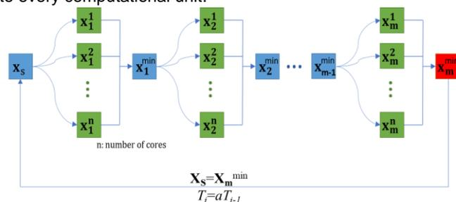
Figure 2: Synchronous parallel simulated annealing algorithm architecture.
