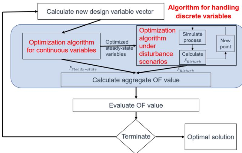
Figure 1: Generic solution procedure of the approach, invariant of the algorithms used.
