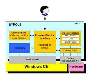
Figure 1. System architecture
