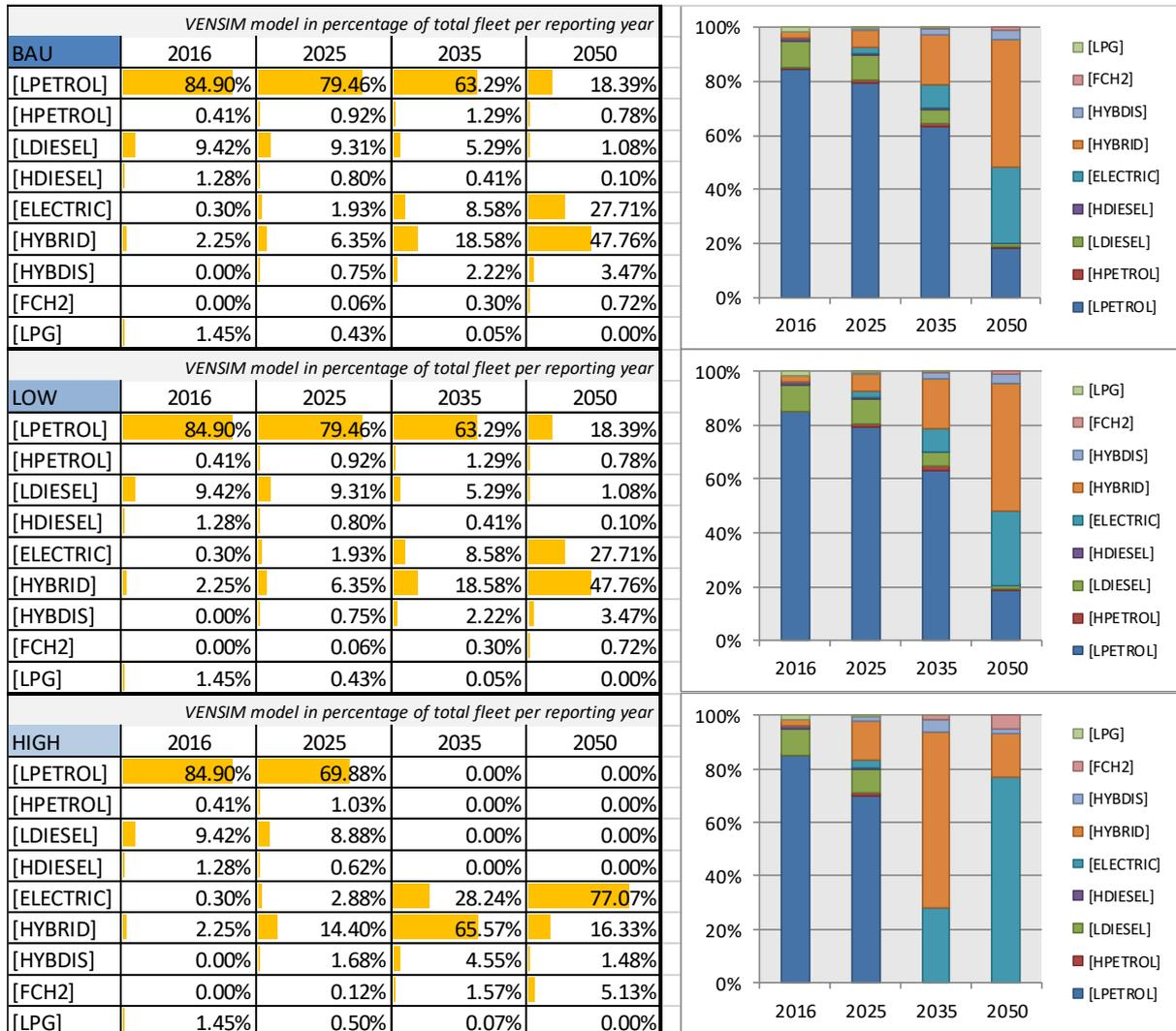
**Figure 3-6: Passenger car fleet composition in the BAU and in the Low and High (and Final) Scenario. Since the fleet component of the Final Scenario is the same as the one of the High Scenario, the bottom row also corresponds to the Final Scenario.**
