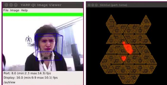
Fig. 1: Extracting facial features from iCub’s cameras and tactile information from the skin on iCub’s torso
