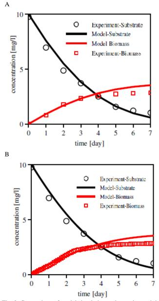
Fig. 2. Comparison of model simulation and experimental data before (A) and after (B) parameter estimation
