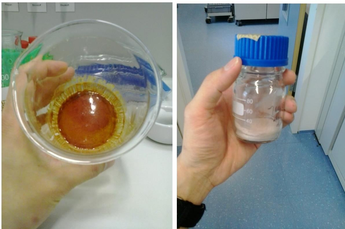
**Figure.** “Purified peptone” before being redissolved in water (left), and final protargol powder product (right).
