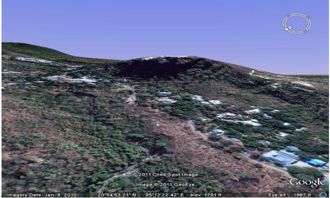
Figure 8. Satellite image showing foot slope of Taunggalat which is gently inclined away from the centre and talus debris materials
