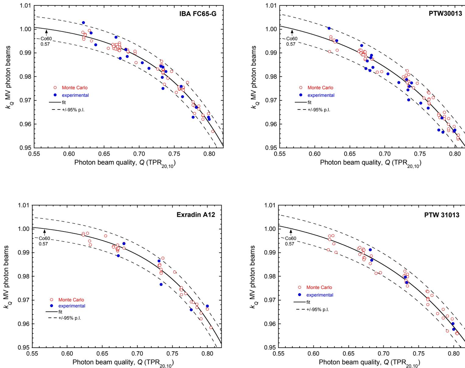
Figure 2: Values of  $k_Q$  for megavoltage photon beams obtained from Monte Carlo calculations by different research groups (open circles) and measured at primary laboratories (filled circles) for the Farmer-type chambers IBA FC65-G, PTW 30013 and Exradin A12, and the PTW 31013 Semiflex chamber type. The solid lines are fits to the combined data set using Eq. (6) and the dashed lines are the 95% prediction limits of the fit.
