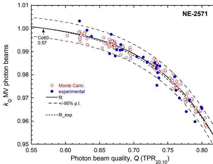
Figure 1: Values of  $k_Q$  for megavoltage photon beams obtained from Monte Carlo calculations by different research groups (open circles) and measured at standards laboratories (filled circles) for a NE-2571 Farmer-type ionization chamber. The solid line is a fit to the total of 154 data points using Eq. (6) and the dashed lines are the 95% prediction limits of the fit. The short-dashed line corresponds to the fit of the 28 experimental data points.
