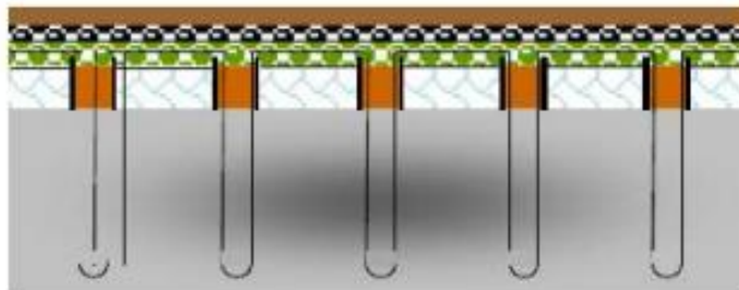
Borehole thermal energy storage (BTES) (15 to 30 kWh/m 3 )
