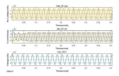
Figure 9. Line voltage of transformer primary, wind generation load current and line voltage of transformer secondary
