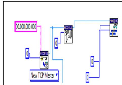
Fig. 3. Representation of Meter Data Addressing
