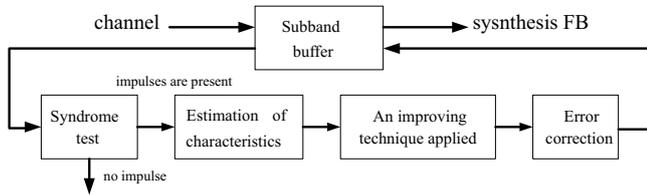
Figure 2: Error correction scheme
