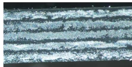
**Fig. 5.** Microscopy picture of the laminate section manufactured with the new thermoplastic material
