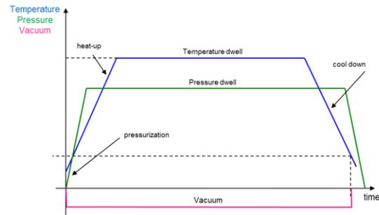
**Fig. 4.** Autoclave consolidation cycle
