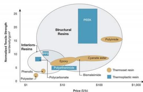
**Fig. 1.** Normalized Tensile Strength vs. Raw Material Price for Aerospace Thermoset and Thermoplastic polymers [5]
