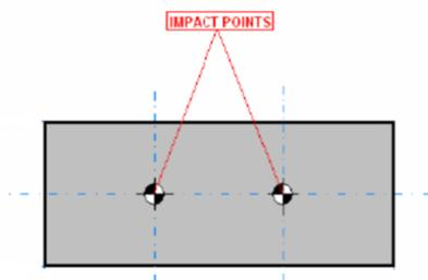
Fig. 8. Hail impact test element
