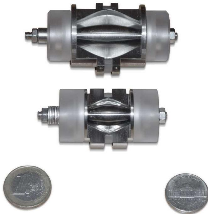
**Figure 7.** Cut-outs of a standard (top) and a high-field (bottom) Orbitrap analyzer (reprinted with permission of Thermo Fisher Scientific, CCL2012).
