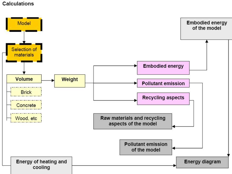
**Figure 5:** Calculations flowchart.
