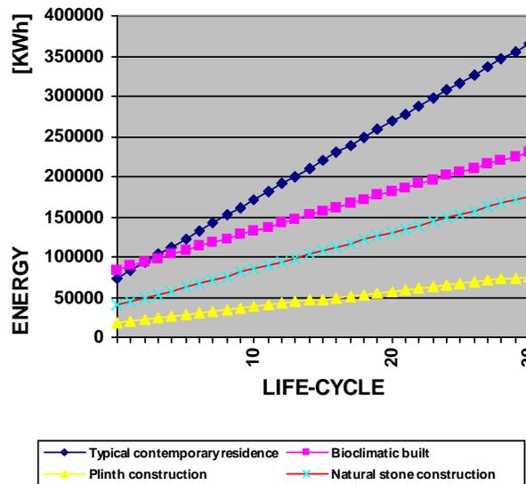
Figure 8: Energy evaluation diagram
