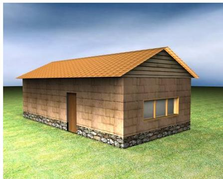
**Figure 3:** Model 3. Plinth construction
