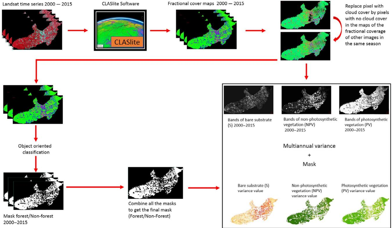
**FIGURE 2** CLASlite software processing of Landsat images for the assessment of photosynthetic vegetation, non-photosynthetic vegetation, and bare substrate (S) bands in a multiannual period, and non-forest mask building from CLASlite results [Colour figure can be viewed at [wileyonlinelibrary.com](http://wileyonlinelibrary.com)]
