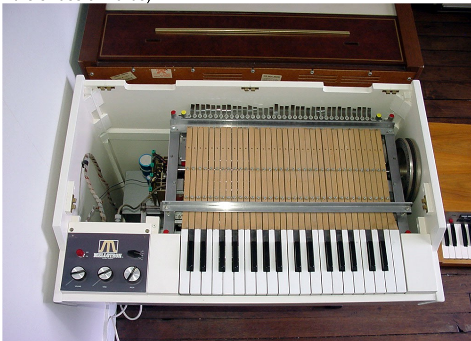
Fig. 2 M400 mellotron, with 35 keys, 35 magnetic tape strips and inner motor mechanism.
