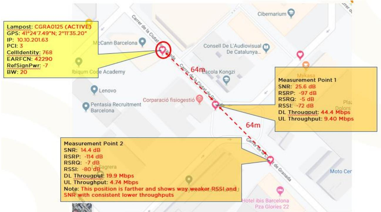
Figure 10: 5GCity Small Cell CGRA0125 initial throughput at range validation
