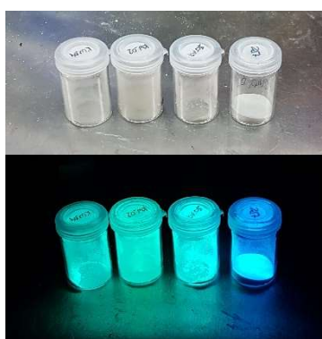
Figure 3: Photographs of \text{ASr}(\text{BH}_4)_{3-x}\text{Cl}_x ( A = \text{K}, \text{Rb}, \text{Cs}; x = 0.20, 0.14, 0.26 ) and \text{Sr}(\text{BH}_4)_{2-x}\text{Cl}_x ( x = 0.26 ) from left to right. Top: Samples under daylight, bottom: Samples under 365 nm excitation in an argon filled glovebox.
