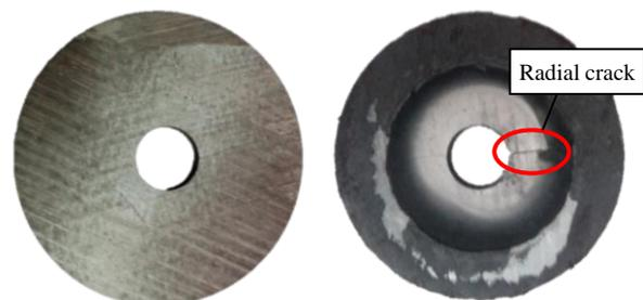
Fig. 8. Pictures of the CI-LF-1 chamber insert before and after test.
