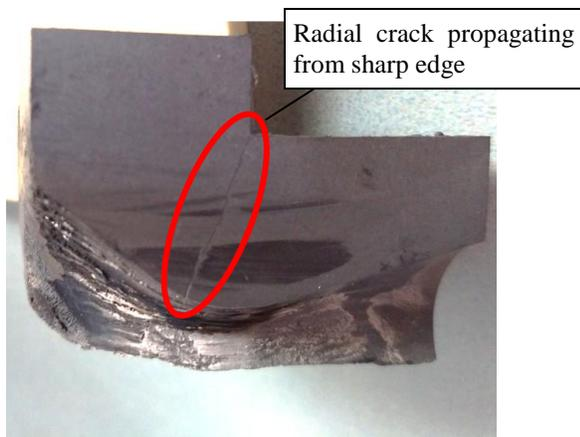
Fig. 19. Picture of the cut section of CN-SF-1 nozzle correspondingly to the radial crack.
