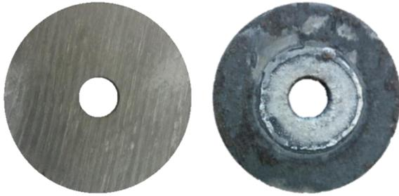
Fig. 9. Pictures of the CI-LF-2 chamber insert before and after test.
