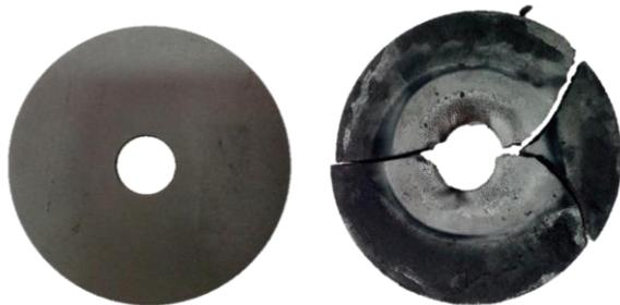
Fig. 10. Pictures of the CI-SF-1 chamber insert before and after test.
