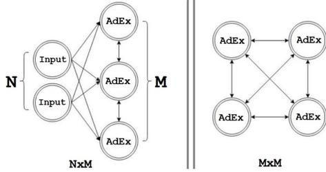
Fig. 1. Two types of network setups examined by the simulator. A layer of  $N$  spiking neurons feeds a layer of  $M$  AdEx neurons ( $N \times M$  case); or  $M$  AdEx neurons form interconnections and interact with one another ( $M \times M$  case).
