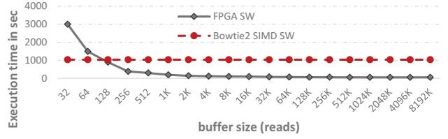
Fig. 8: Impact of input buffer size on accelerator-call overhead and thus execution latency.
