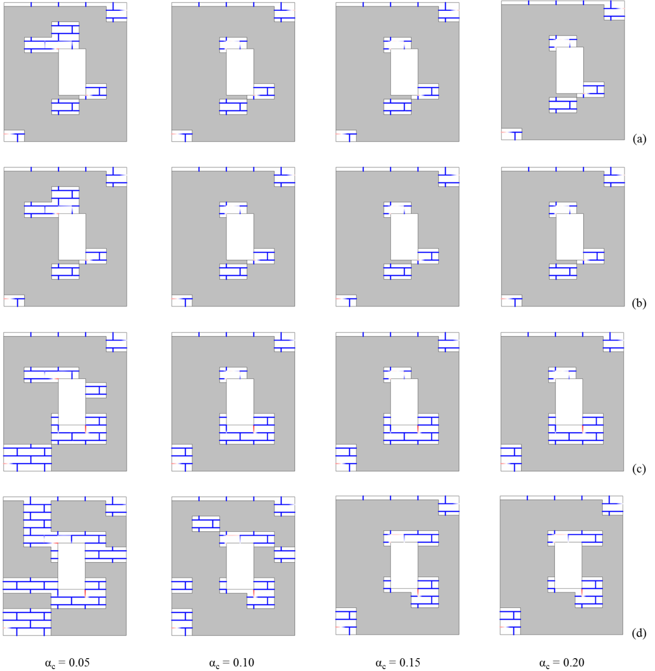
Fig. 14. Damage variable maps for \delta = 0.25 mm obtained from the multiscale numerical simulation (MNS) performed for different values of both the tolerance parameter \alpha_c and the scale factor c : (a) c = 1/1.5 ; (b) c = 1/2 ; (c) c = 1/3 ; (d) c = 1/5 ; the coarse-level elements outside the zone of interest are shaded in grey, whereas the damage variable defined on the cohesive interfaces ranges from 0 (blue) to 1 (red).
