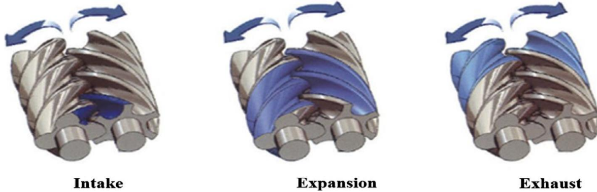
Figure 10: Working general design and principle of a screw [40]
