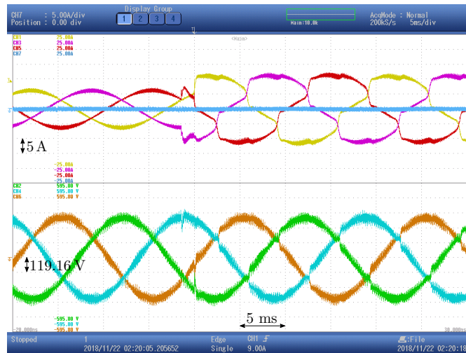
Fig. 11. Transient-state from Test 1 to Test 2. Top: i_{s,a} (yellow), i_{s,b} (purple), i_{s,c} (red) and i_{s,n} (blue). Bottom: v_{s,an} (green), v_{s,bn} (light blue) and v_{s,cn} (orange).
