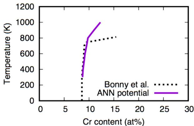
**Fig. 7.** Phase diagram for the FeCr binary alloy, as predicted with Metropolis MC based on our rigid-lattice NNP. The dashed line is a review from experimental data in Ref. [37,38]
