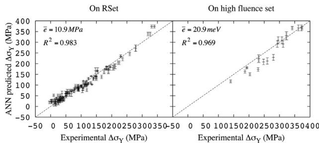
**Fig. 4.** ANN quality of prediction of the neutron irradiation induced increase  $\Delta\sigma_Y$  in the yield stress of RPV steels. The number of input variables is 4, and the number of hidden nodes is 4. Error bars show the standard deviation of predictions made by 25 different ANN, trained with the same training and reference sets. (left) Prediction on the reference set. (right) Prediction on a separate set that corresponds to higher neutron fluences, that was not used for training.
