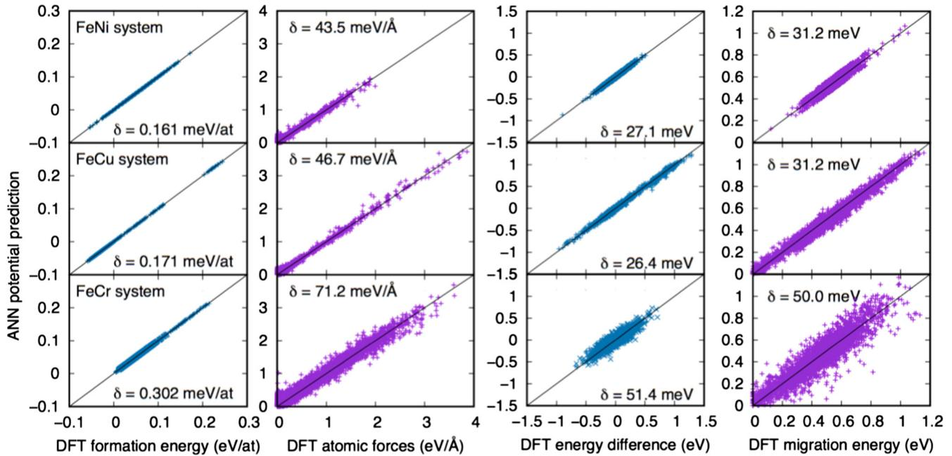
**Fig. 6.** Accuracy of prediction achieved by the ANN potential while reproducing NEB calculations for evaluating the saddle point during the migration of single point-defects (either a single vacancy or a single SIA) in binary bcc alloys.  $\delta$  is the mean absolute error of prediction.
