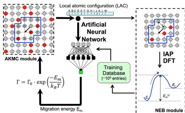
**Fig. 8.** AKMC model aided with ANN for fast and accurate on-the-fly estimations of the activation energies associated to the migration of single point-defects.
