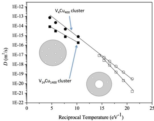
Fig. 12. Example of Arrhenius plot computed with the ANN-based AKMC for the diffusion coefficient of Vac-Cu clusters.
