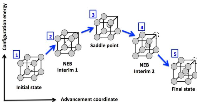
Fig. 5. Atomic configurations extracted from NEB calculations (vacancy migration event) with DFT, used to design an ANN-based potential.
