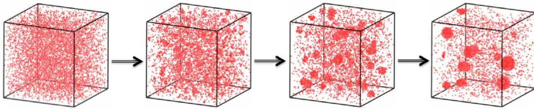
Fig. 10. Snapshots from an AKMC simulation of a thermal annealing experiment in a Fe-1.34%Cu at 500 °C.
