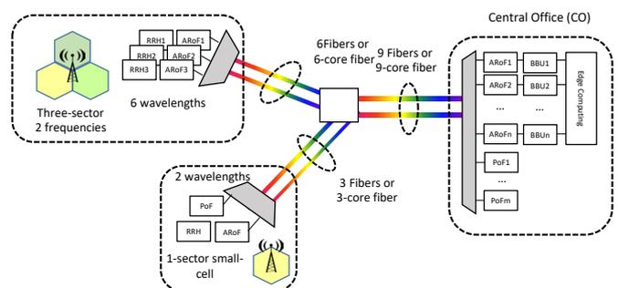
Fig. 1. Proposed optical fronthaul architecture
