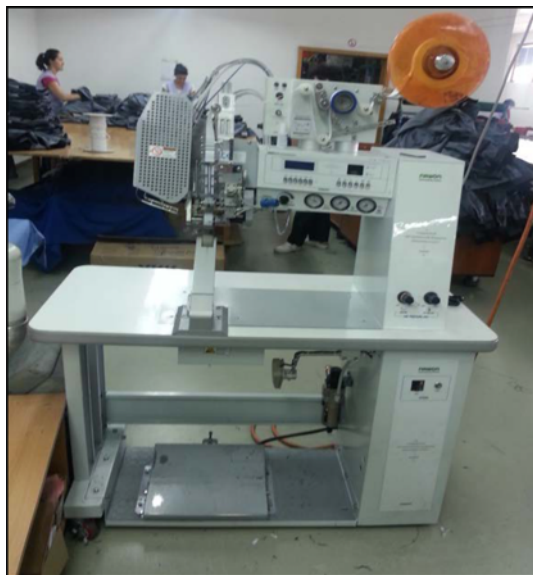
Figure 3. Hot air seam sealing machine NAWON.
