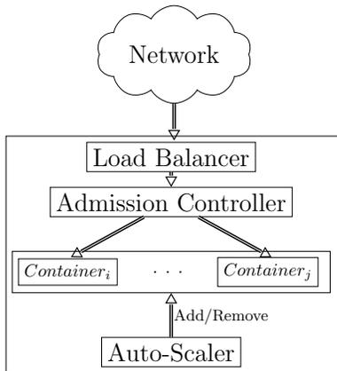
Fig. 2. Proposed container auto-scaling architecture.
