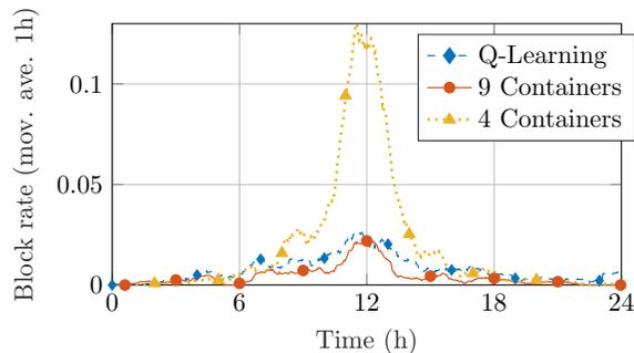
Fig. 6. The blocking rate observed over the time during Docker experiments in terms of rejected requests per second.
