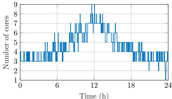
Fig. 5. Scaling decisions taken by Auto-Scaler algorithm during the Docker experiment at 20% of convergence (using  $\beta = 0.02$ ).
