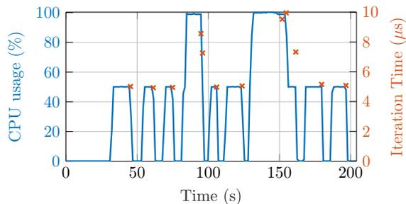
Fig. 3. Relationship between CPU utilization and service time. When reported utilization is  $\leq 50\%$  iteration time is predictable.
