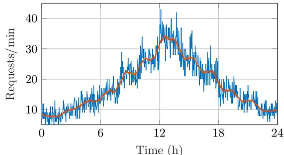
Fig. 8. Traffic profile observed during the Kubernetes experiments. Traffic rates are taken over two-minute windows. The red line is the moving average over 30 samples.
