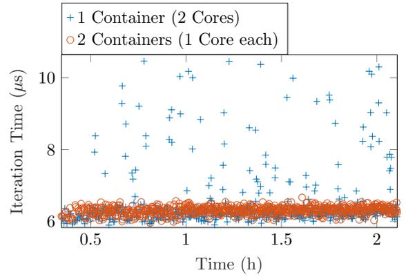
Fig. 1. Vertical vs. horizontal scaling: two containers running on distinct cores provide more predictable performance than one container running on two cores.
