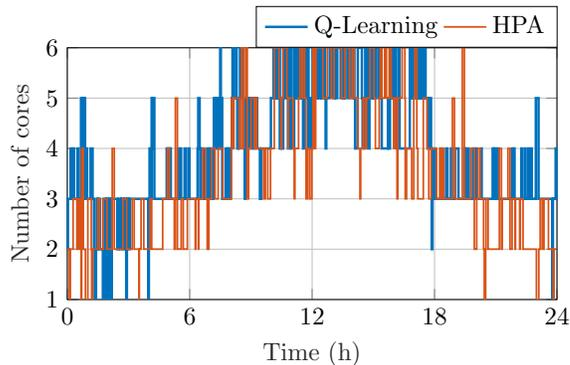
Fig. 9. Scaling decisions taken by the AS algorithm during the Kubernetes experiment at 25% of convergence (using  $\beta = 0.02$ ).
