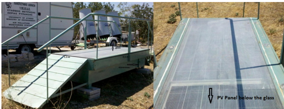
Fig. 5. Photovoltaic pavements (Efthymiou et al., 2016).
