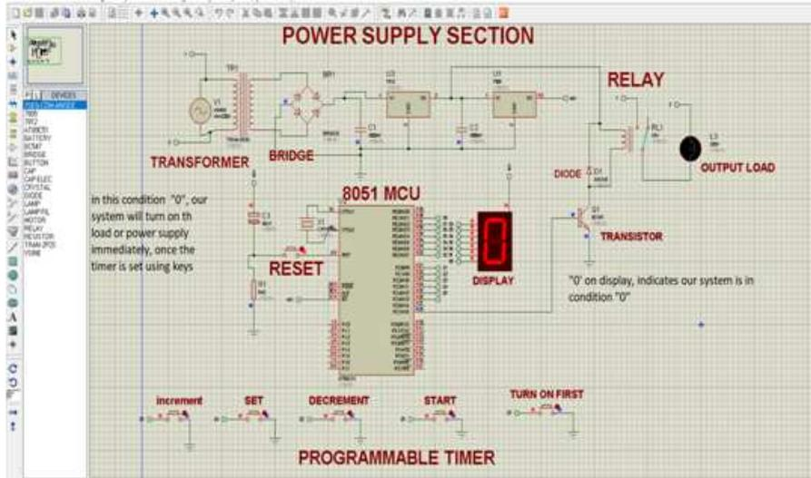
In this condition "0", our system will turn on the load or power supply immediately, once the timer is set using keys
