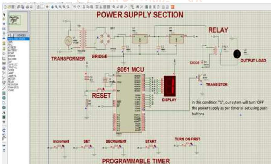
In this condition "1", our system will turn "OFF" the power supply as per timer is set using push buttons.
