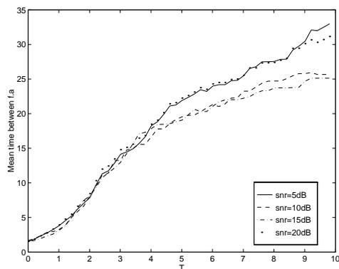
Figure 4: Mean time between false alarms as a function of the threshold
