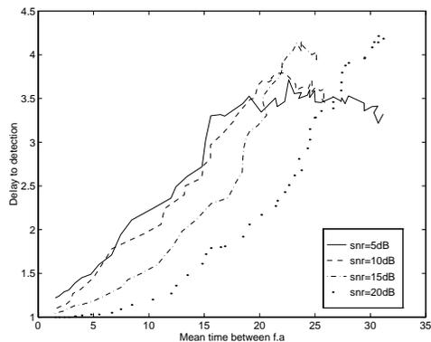
Figure 5: Delay to the detection as a function of mean time between false alarms
