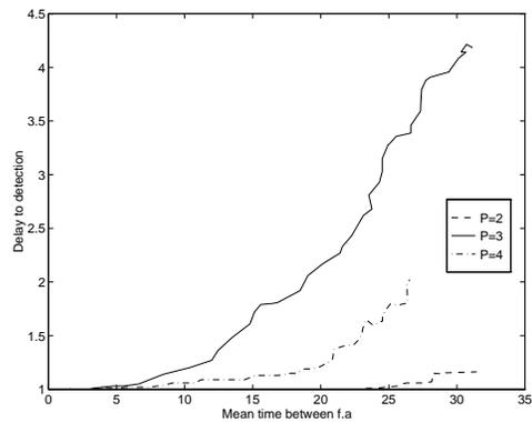
Figure 7: Delay to the detection as a function of mean time between false alarms
