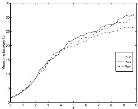
Figure 6: Mean time between false alarms as a function of the threshold
