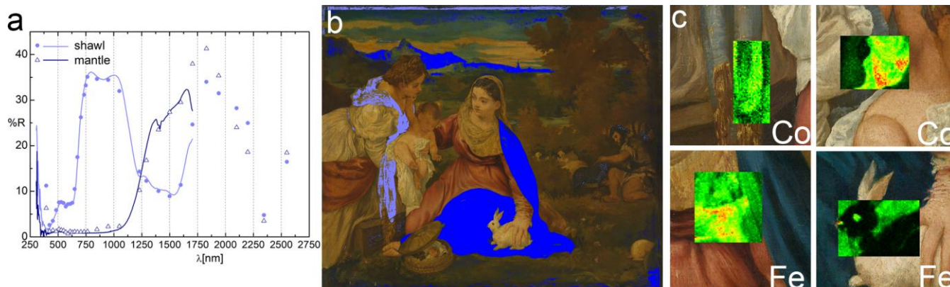
Figure 3. Manet: a) FORS (full line) and scanner (dots, triangles) reflectance spectra of blue shawl and mantle, b) SCM of blue pigments: Cobalt blue codified in periwinkle, Prussian blue in electric blue colour, c) XRF Co and Fe maps as referenced on 10x10 cm areas.
