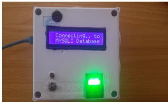
Figure 8: LCD displaying connection status between the Arduino and the database
