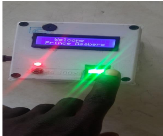
Figure 7: Fingerprint based system welcoming user after successful identification
