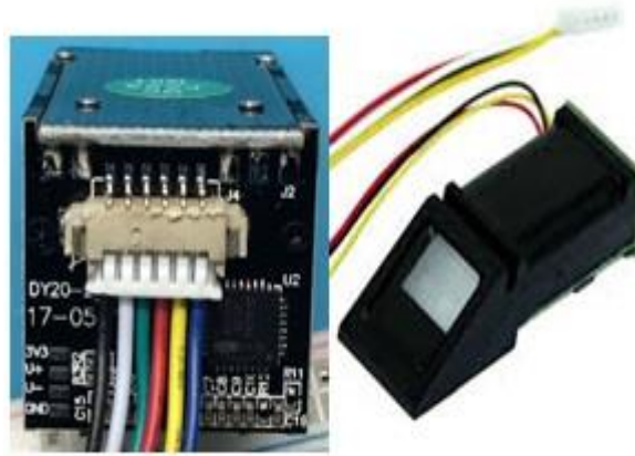
Figure 4: Front and Back image of Adafruit Fingerprint Reader DY50
