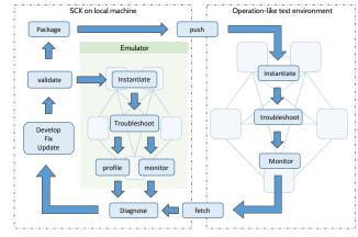
Fig. 4: SCK Workflow for network service development.
