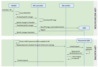
Fig. 2: Specific Manager instantiation and runtime sequence diagram.
