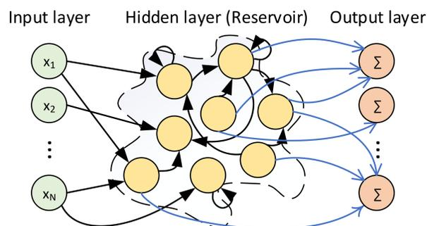
General schematic of a reservoir computing. The blue arrows are the only weights trained.
