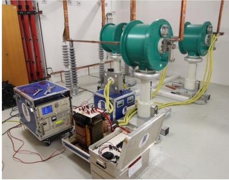
Figure 4: Pictures of an actual on-site LMS component calibration of the current channels (left) and voltage channels (right), using a sampling current ratio bridge and a high-voltage capacitance bridge [19, 20].
